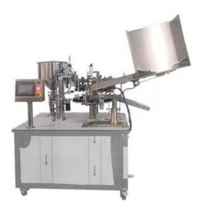
This machine is mainly used for quantitative filling and sealing of Aluminum Tube Metal Tube composite hoses as packaging container materials. This machine is widely used in packaging in medicine, daily chemical, food, chemical and other industries.
