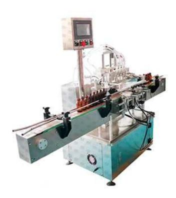
Our automatic linear structure vacuum liquid filling machine is a machine that first pumps air to the packing container to form negative pressure, and then fills the liquid into the packing container.
