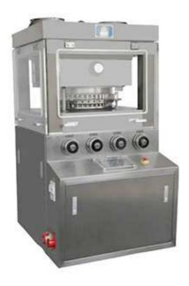
Double-pressing type and single-sided tablet discharging. It uses ZP punch to press granular raw materials into round tablets and special-shaped tablets of various specifications.
