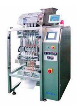
The high speed multi-filed bagging accomplishes bag forming, counting, filling, bag sealing and printing at the same time. Counts by infrared and sensor that doesn't wear or break the product and is compatible with all kinds of materials.
