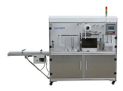
The Stretch-Banding Machine is an End-of-Line Packaging Machine. It can group together or stack cartons (or similar shaped objects) to form larger units. These are then tightly wrapped in plastic film. Compared with shrink-wrapper and overwrapper, this machine is energy-saving as it does not require heating up. It saves 50% of film materials because it partially covers the packaging. It can be connected to a packaging line with Blister Machines, Cartoners and Case Packers.
