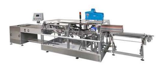
The VDC-2900 is a versatile machine that can run regular, tuck and gable top cartons. VDC-2900 has two, manual loading stations where product is manually loaded by operators. Hand load area can be extended to accommodate up to 10 operators. For high speed applications, VDC-2900 can be upgraded to fully automatic.
