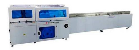
Sealing Machine ZF-BS500-Z provides customers with fast packaging solutions, with a packaging speed of 80-120 packages per minute. It can meet different specifications of products and packaging mode, the conversion process is convenient and fast. Excellent in flexibility and stability, the edge sealing machine is especially suitable for customers who need to deal with different types of products frequently.
