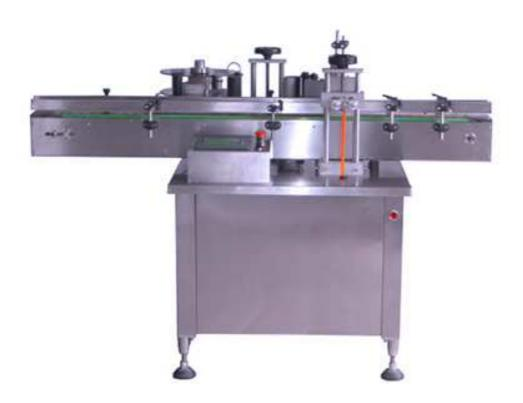
OLR-V is economical, self contained, easy to operate, equipped with auto teach programming touch screen. Built in microchip storing different job setting makes fast and easy changeover. This automatic labeling system can orient label precisely for cylindrical container.
