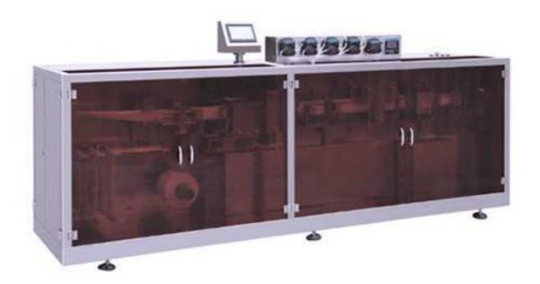
Take out the film, Plastic bottle-forming, filling, date printing, sealing and cutting can be completed automatically. Save cost and time.
