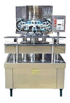
ZPC-12 Auto-bottle rinsing machine adopts the high technology from aboard, by adopting gyration method on rinsing device, it can automatically complete working process from bottle entry, bottle rinsing, water removing to sanitize bottle out. It is most advanced and suitable device to rinse the bottles made of PET or glass bottles. It can become a complete auto-product line if it works with filler and sealer together.
