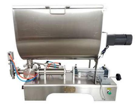
The LT-500U mixing sauce filling machine material valve control system adopts the unique patented technology. It could do the filling of solid material containing chunk, semi-liquids and dope, and the sauce of oil, water, material in separation condition. The liquid contractive parts are made of stainless steel, meeting GMP requirement.
