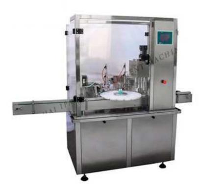
Vial Liquid Filling and Stoppering Machine is suitable for the liquid filling and rubber stoppering of glass vials. Machine complete in pleasing matt finished stainless steel construction. The basic unit consists of turntable/unscrambler, SS Stat conveyor belt, Highly efficient and precision built S.S. 316 Syringes, non- toxic synthetic rubber tubing and easy reach compact panel.
