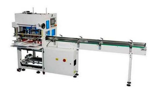
Cylinder packaging machine ZF-X450, The adjustable push plate is suitable for packing products of different widths. The packing speed can reach 20 barrels per minute. It is suitable for the whole package of OPP sealing tape, stationery tape and PVC electrical tape.
