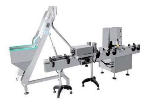
This machine is used for capping glass jar which contained condiments, beverage and so on. After equipped with vacuum system, the machine pumps air to make the glass jar into vacuum state, and then seal with screw cap. It could prolong the shelf life and improve the mouth feel. It is automatic jar-in, automatic cover down, no-jar-no-cover and vacuum function.
