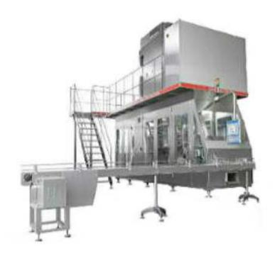
It applies to sterilization by liquid UHT milk and a variety of non-carbonated drinks, fruit juice, coffee, plant protein drinks, tea drinks, wine etc. gravity of aseptic packaging of liquid food, the machine uses all stainless steel materials, core components All of a world-class brand, auto-complete feed, sterilization, filling, forming, packaging in the form of paper aluminum composite brick.
