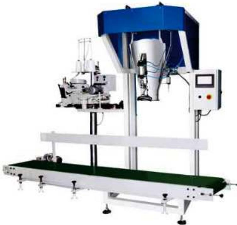
It's suitable for weighing corn, soybeans, rice, barley, wheat, buckwheat, peanuts, beans and other small granules in food industry, light industry, chemical industry in bulk weight.
