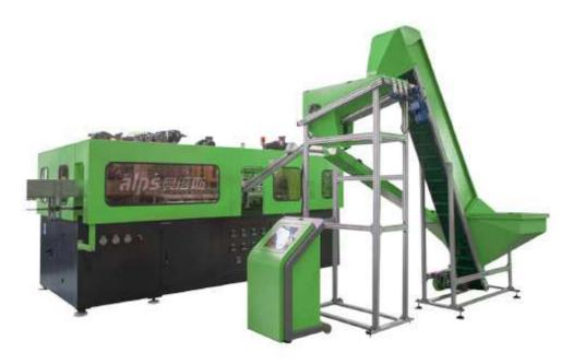
The two-step Pet stretch blow moulding machine which are applicable in a wide range of PET packaging practice, such as for beverages, edible oil, food, pharmaceutical products and cosmetics, etc. With more than 10 years experience in developing and producing blow molding machine as well as the advanced technology absorbed domestic and abroad, we have developed with our constant innovation dozens of high speed and high precision equipments which have won the top reputation in the field.
