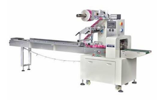
This vegetable packing machine is use for vegetable and fruits. The packing speed of vegetable packing machine can up to 200bags one minute. It can work with the metal detector. Stable quality, reasonable price, long time good sell-service make us gain many customers all over the world.
