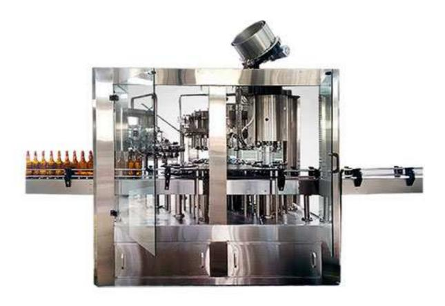
The 16 heads filling machine designed by HEM Company adopts the Counter pressure filling technology which can perfectly realize the requirements of twice vacuum, CO2 injection (pressure preparation). The machine also adopts 3 in 1 compact design, easy to operate and maintain.
