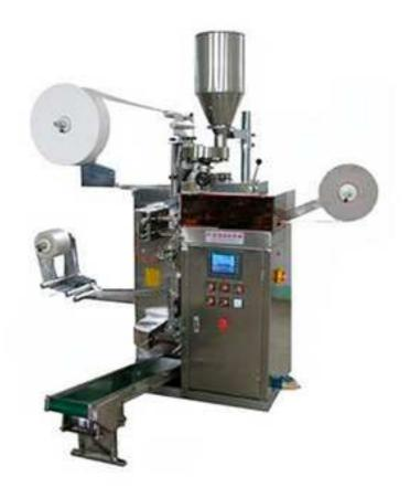
This machine is suitable for green/black tea, medical tea packing, inner bag and outer bag was forming at one time.
