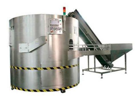
JLP-2000 serial full-automatic bottle unscrambler is the support equipment for the soft beverage filling equipment, applicable for the orderly arrangement of messy PET bottles and the delivery of them to production line.
