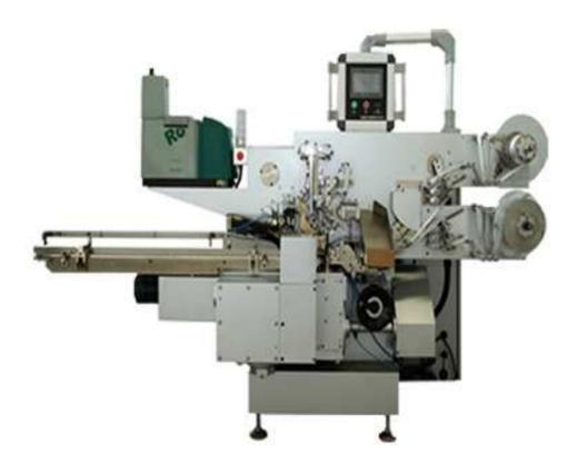
Folded Packing Machine is the fully automatic packing machine which can be used for chocolate, pralines and pressed candy Machine is suit for small-to medium dimension products with certain dimension and shapes packing in the fold style (also available for additional label wrapping). The maximum packing speed is 450 pieces per minute, which can vary according to different product shapes and packaging materials.
