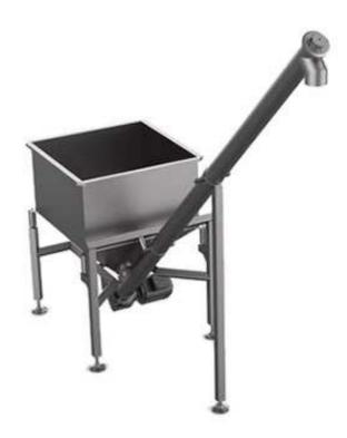
This is inclined screw elevator applied to transport powder product from one station to the other! The conveyor is designed with a U-Shape trough and a cap on the trough hinged by buckle with good sealing in the middle, easy for opening or cleaning.
