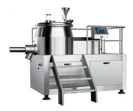
In the cylinder (conical) container, powder materials and binder will be mixed into moist soft materials by the mixed paddles at the bottom. Then they will be cutter into uniform wet-particles by the side high-speed smashed paddles.
