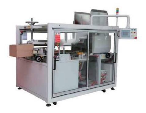
The carton storage adopts the horizontal type, and the empty carton can be refilled at any time, without stopping the machine, saving and opening the door safety protection function, the door is opened and the machine pauses and alarms, and the indicator light flashes.
