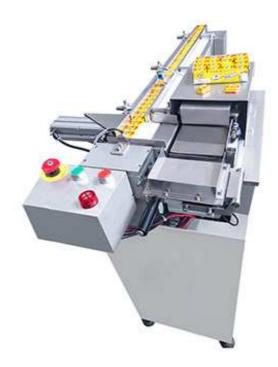
The machine is our new design, it's suitable for boxing cubes, medicine, cosmetics, and goods etc. It is a semi-automatic multi-layer boxing machine. After the products are arranged, the cylinder will push them into the mold to complete the arrangement.
