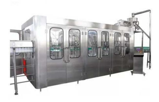
Automatic orange juice hot filling machine for PET bottle. The standard type of RCGF series hot filling machine is "4-in-1", aiming at special production condition, one disinfectant rinser can be increased to be 4-in-1 monobloc. The system gives full consideration for beverage's characteristics (e.g. it is easy to have foaming for tea beverage and mixed juice.) and main technical requirement of hot filling.
