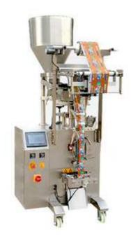
The small vertical multi-function packaging machine adopts PLC control touch screen operation. The equipment is equipped with automatic measuring device for measuring cups and chain bucket mechanism for manual weighing and feeding. The two methods can not only meet the automatic measuring of uniform materials, but also meet the packaging of materials that are not suitable for automatic measuring.
