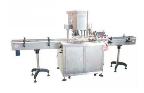
This machine is suitable for packaging various round cans, such as tin cans, aluminum cans, plastic cans, and paper cans. The machine has two pairs (four) of wheel seam seals. To seal round cans of different specifications, you only need to replace the pressure head, turntable, and lower cover device. High production capacity, wide application range, high degree of automation and easy adjustment. Suitable for canning production line equipment.
