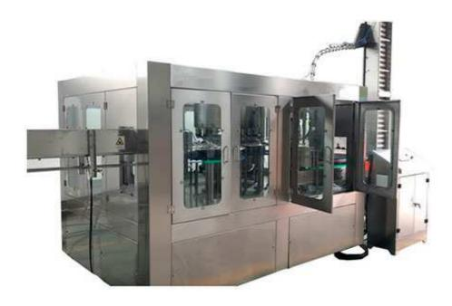
Bottled Drinking Water Filling Machine, Its Filling Method Is Gravity Filling. Gravity Filling Machine, Also Known As Atmospheric/Normal Pressure Filling Machine, Means That Under Atmospheric Pressure, It Directly Relies On The Weight Of The Filling Material To Flow Into The Packaging Container. This Kind Of Filling Is Only Suitable For Filling Liquid With Low Viscosity And No Gas.
