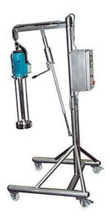
PMS HOMOGENIZING MIXER® provides high-shear agitation to moderately low-viscosity fluids. The homogenizing mixer is used to prepare suspension or emulsion. The test result obtained from laboratory unit assures a reliable scale-up to the larger production units.
