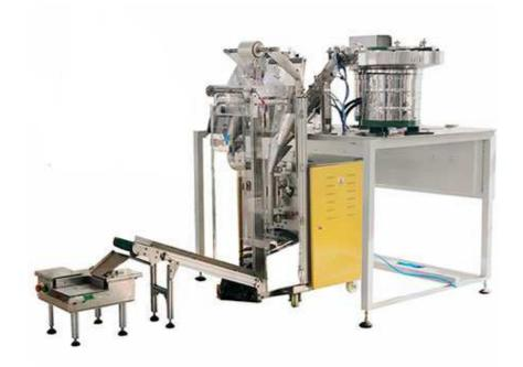
This machine is applicable to single items packing and mixed 2-3 types of items packing, operating easily with PLC control system. Firm sealing, smooth and elegant bag shape, high efficiency and durability are preferred elements. Automatic ordering, counting, packing and printing can be offered. Equipped with exhaust device, printer, labeling machine, transfer conveyor and weight checker make it better.
