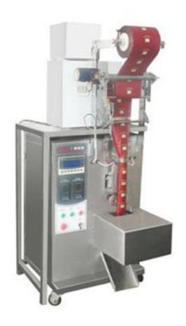
The MK-T60 vertical form fill seal machine is equipped with a microelectronic scale to guarantee packaging accuracy, making it applicable to the automatic packaging of black tea, herbs and other items. The MK-T60 machine features an automatic weighing, automatic bag making, sealing, and cutting performance.
