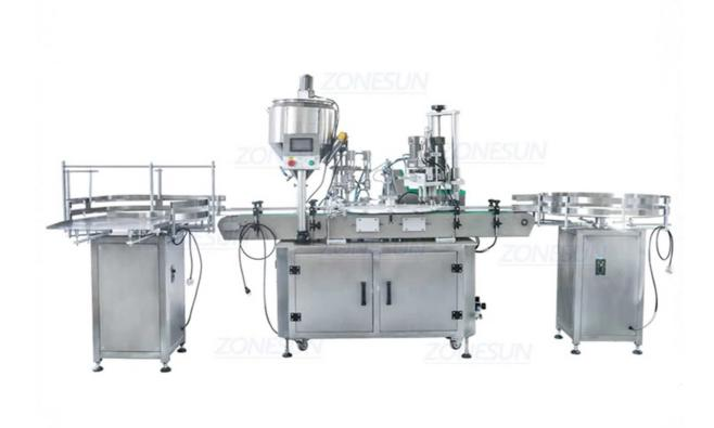
This automatic production line is designed with multiple function, it can arrange bottles, fill liquid or paste, feed bottle caps, cap bottles and sort finished products automatically. It can help you improve working efficiency. This is suitable for essential oil, water, juice etc. We can customize the machine and make it can work for different sizes of containers at the same time.
