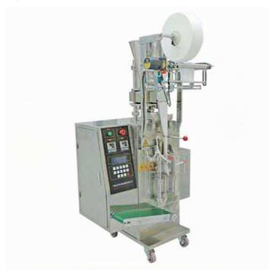
Particle automatic packaging machine is suitable for packaging granular materials such as soup, tea, granule, desiccant, monosodium glutamate, sugar and so on.
