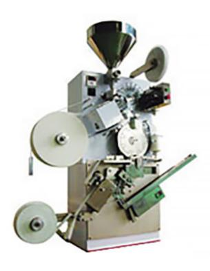
Model CCFD6 Tea bag packing machine features such functions as automatic ration filling, heat-sealing of tea bags, automatic plastering of cotton thread and tags, and cold-sealing of the envelope in the longitudinal direction.
