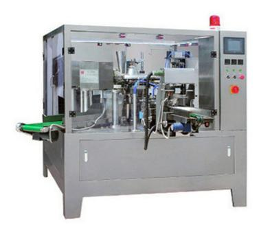
Bag-feeding rotary bag packing machine. The packing materials loss low, what this machine is used the preformed bag, the bag pattern is perfect and has a high quality of the sealing part, this improved the product specification.
