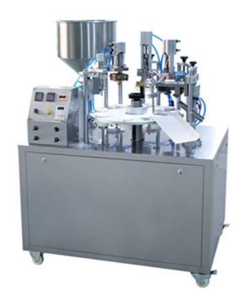
This machine applies the transmission principle. It uses the slot wheel dividing system to drive the conveyor table to do intermittent movement. The machine has 8 or 10 tube stations. Expect manually feeding the tubes onto the machine, it can automatically position the tubes, fill the material into the tubes, heat both inside and outside of the tubes, seal the tubes, press the codes, and trim the tails and the finished tubes exit.
