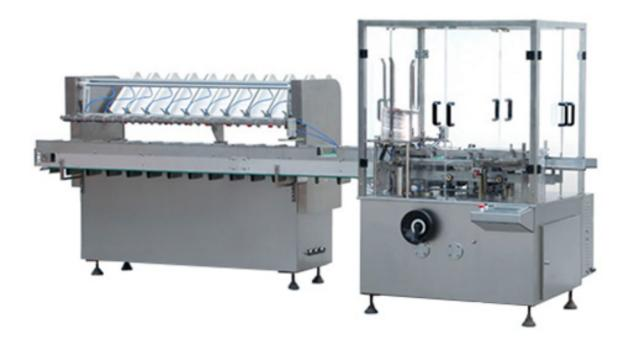
This machine is suitable for scratch, punch, soft al/al strips, wound paster, ointment plaster, facial mask, coffee bags into carton automatically. On line product feeding and detecting, carton opening and forming, products and leaflet pushing into carton, printing batch number, sealing carton with tuck-in or hot melt glue device. Automatically reject lacking of leaflet or product and finished product out.
