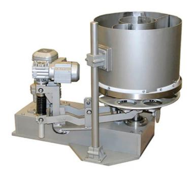
Automated systems, like the Volumetric Cup Dosing Filling Machines, have been developed to enable accurate measurement and distribution of specific amounts into containers. The core of these machines is the volumetric cup concept used for measuring the volume of a desired product.
