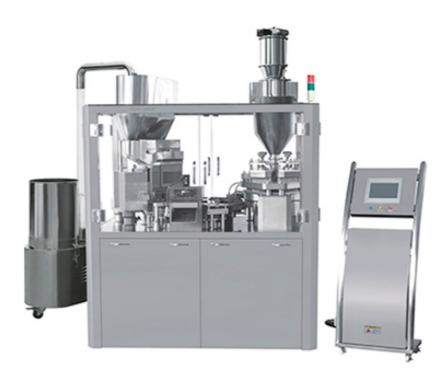
Auto Capsule Filling Machine is used to fill powder in the form of slug in hard gelatin capsules.
