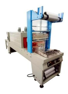
The product can be fed manually or pneumatically. When the sealing & cutting cycle is complete, the product is discharged into the shrink tunnel automatically. The machine is used to shrink package single and multiple products.
