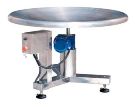
Mainly used to collect the finished bags from packaging machine for more packaging steps, normally connected with packaging machine and take away conveyor. Machine made of 304 sanitary stainless steel, with inverter for variable speed. With fast installation and assembling.
