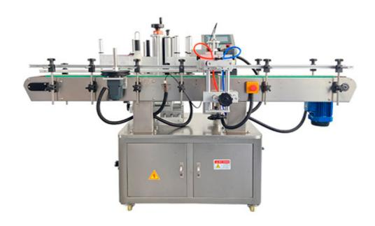
This automatic labeling machine is suitable for sticking labels on round bottles, plastic bottles, glass bottles, etc. It can be used for single side or double sides labeling, improving work efficiency. Adopting the way of positioning and labeling, it can label bottles accurately. The machine can be widely used in pharmaceutical, cosmetic, beverage, daily chemical industries.
