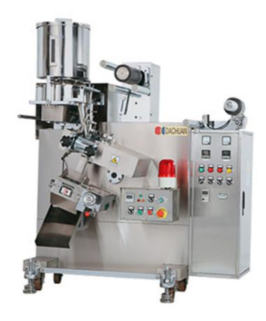
The DC-338 series machinery is a roller-type packaging machine for automatic forming, filling, and sealing of liquid, viscous (cream, sauce, etc.), powder, and granular materials. This machine can achieve three-side or four-side sealing packaging.
