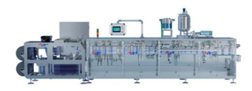
This machine can realize the packaging needs of straight nozzle bags, and can also add hanging holes, special shapes, zippers, nozzles and other functions, realizing automatic bagging, automatic filling, automatic nozzle addition, automatic nozzle welding, and automatic sealing. It is used in the packaging of salt, lubricating oil, beverages, juice, yogurt, sauces, edible oil, and cleaning series.
