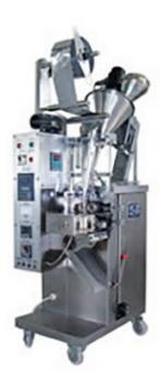
This powder packing machine is mainly used in the automatic soft-bag packaging of powder materials in fields of food, pharmacy, chemicals, etc.
