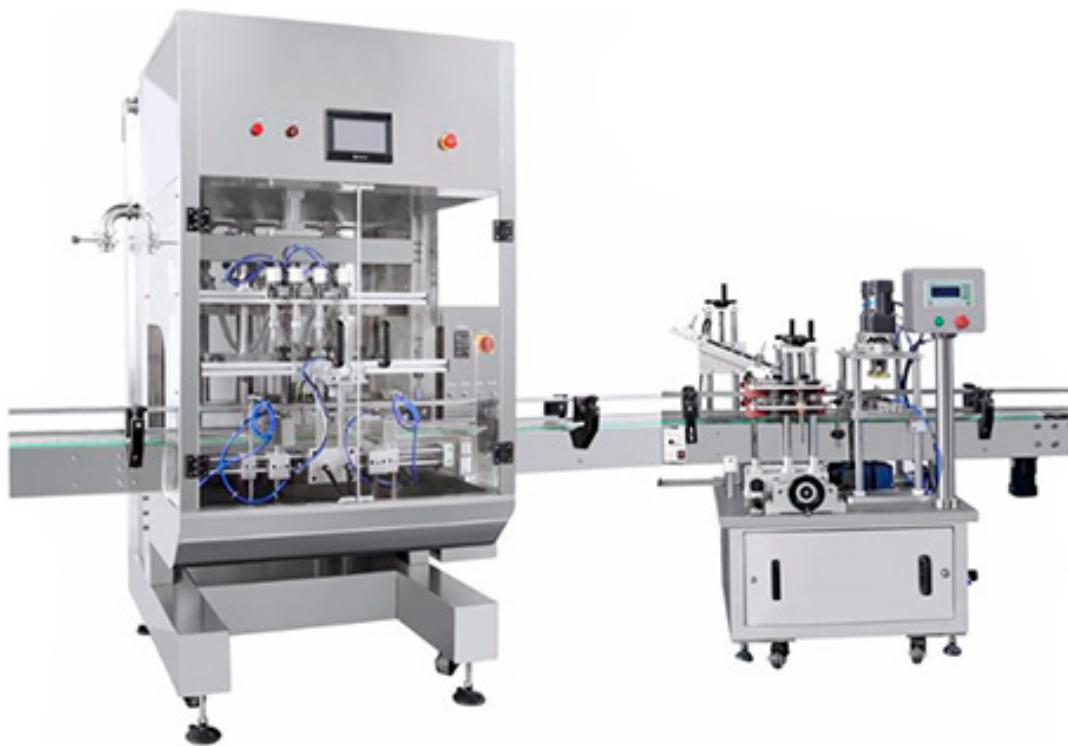
This line consists of bottle/jar feeding table, weighing filling machine, cap feeding machine, capping machine, labeling machine, etc. used for filling liquid/paste into bottle or jars.
