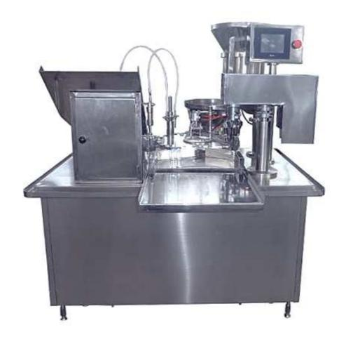
This machine is the filling apparatus in the oral liquor assembly line, which is mainly applied in filling, lading, screw sealing of 2 - 30 ml bottles. The operation of filling and sealing is combined in this machine with its advanced design and compact structure. There are two filling nozzles on this machine, guarantee the filling is smooth. This machine can customized according to customers' specific request.
