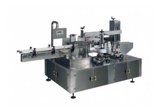
Labeling machines are applied to various operations such as sticking a label on plane, post surface, single side or multi-sides of a package, sticking labels covering part or all of the surface of a cylinder, or sticking on sunken locations and at edges or corners.
